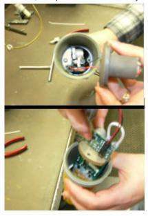
• If the electronic module must be removed/replaced proceed as follows: Remove LED components as described above then locate and remove the two screws attaching the electronic module to the housing and remove the electronic module
