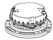
Figure 19: Removing gasket
