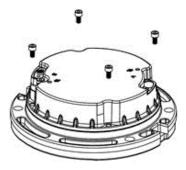
Figure 18: Lifting up housing
