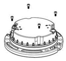
7. Check the light fixture for water-tightness.
