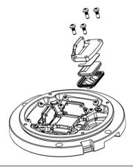
Figure 42: Remove prism and gasket
