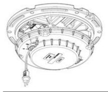
Figure 12: Tighten screws
