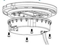
Figure 16: Tightening screws
