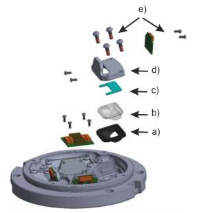
2. Detach and remove the LED board holder, including 4 screws from the body, using a 3 mm Allen key. See Figure 41.
