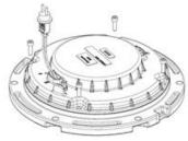
Figure 7: Lift up housing
