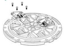
Figure 35: Remove prism and gasket
