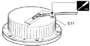
3. See Figure 10. Remove the six screws (E10). The use of an impact driver may be required to unlock the screws.
