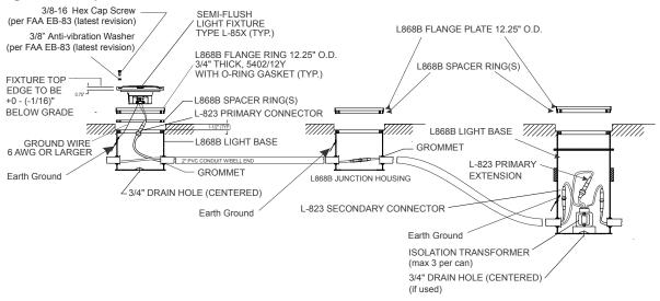
1. Torque according to: FAA EB-83 (latest revision).
