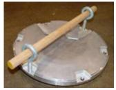
The lifting tool can be made from two  $1/2 \times 13$  eyebolts (1-inch ID) and a 1/2-inch diameter, 16-inch (406mm) long rod or pipe inserted through the eyebolts.
