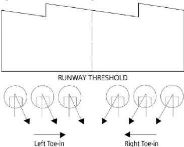
See Figure 3. Refer to the guidelines below for L-850E toe-in coding.
