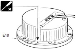
4. See Figure 11. Insert small or medium flat blade screwdriver in the machined recess slot between cover and inner cover and turn it vertically to separate the inner cover from the cover.
