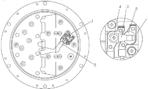
5. Remove installed film disc cutout (2) and replace with the new film disc cutout.
