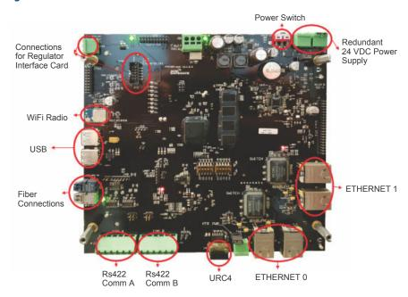
The ACE3 has a connection for interfacing to the Universal Regulator Controller, 4<sup>th</sup> edition (URC4). Connections for interfacing to the Regulator Interface Card (RIC) are provided for controlling and monitoring CCRs that do not contain a URC4 card.
