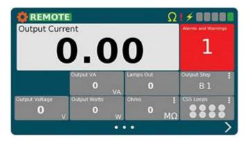
The main screen is the first usable screen (not the splash screen) the user sees after starting the ACE3 (except when in L828 Display mode). The page is laid out with a header at the top and the body below it. The body contains a large display which shows the primary item being monitored.
