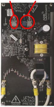
The CVM2 is the latest generation monitoring module. This module is backward compatible with all previous versions of CVMs and can be used as a direct replacement.
