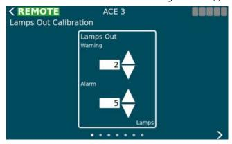
The remaining views act as a wizard. The first three views can be navigated by the user however if the user wishes to start an actual calibration then they must have control of the ACE 3 and they no longer have the ability to navigate through the wizard. They will be allowed to cancel the calibration at any time which will take them back to the first view.
