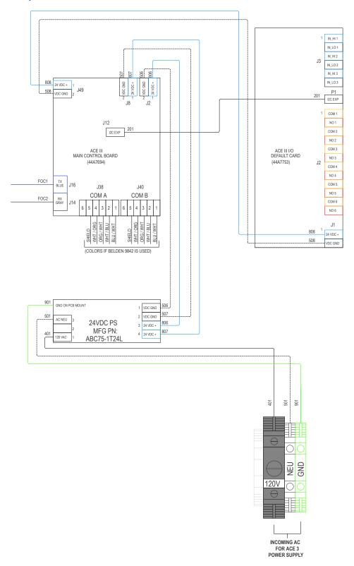
Figure 48: ACE3 power option: 24VDC - 43A4827 5 of 5
