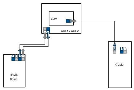
For connections to an ACE3, a dual fiber connection is provided, which will interface to the IRMS board, or directly to the ACE3 main board.
