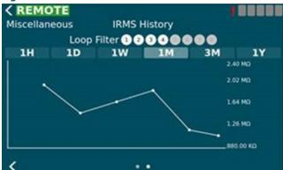
The IRMS History view allows the user to query IRMS data from the past and display it in a graph form so the user can notice trends. The user can select duration of 1 hour to 1 year. If a circuit selector is enabled a loop filter will appear at the top of the view and can be used to filter data based on loops which are being monitored.
