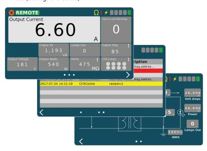
The ACE3 also contains a localized event database to allow the user to view alarms/warnings for the individual device without the need to interface with the higher level control system
