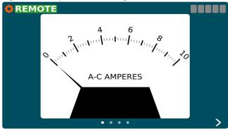
This view is shown when the ACE3 mode is "CCR" and the display mode is L828 or when the "Display Analog Current Gauge" feature is enabled.
