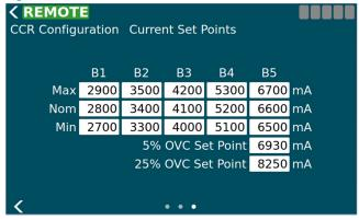
Figure 36: Current Set Point for 20A CCRs
