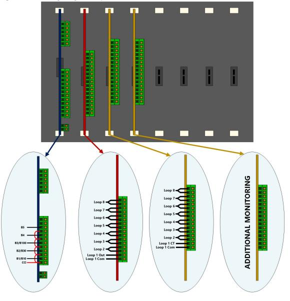
Figure 20: CSS wiring on Integrated CCR using 4x4 Regulator Interface Card
