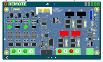
This view is shown when only the 4x4 Regulator Interface Card is installed in a URC4 integrated CCR. The user will have to be in control before they can change the output. Touching an output while not in control causes the "Override Control" popup to be opened asking the user to take control. The board components, LED, and channel indicator on the card will turn red for outputs and green for inputs when activated.
