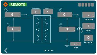
These views are shown when the ACE's mode is "CCR". The first view shows all of the output power related applications. The second view contains input power (if enabled) and output power values arranged on an electrical diagram. If the ACE's mode is "IO" neither the Output View nor the Diagram View will be displayed.
