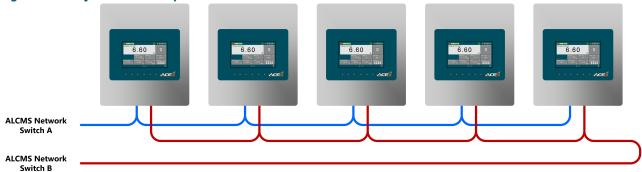
• All ethernet communication cables shall be terminated using RJ-45 connectors using a T-568A Pinout.
