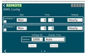
The controls on the scheduling page allow the user to setup the initial delay and the reoccurring interval as well as some additional options.
