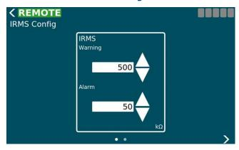
The IRMS config page allows the user to configure thresholds for IRMS alarms and warning as well as set two megging schedules.
