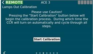
The calibration consists of two phases. The first is calibrating the existing circuit. The second is pulling a set number of lamps and calibrating again.
