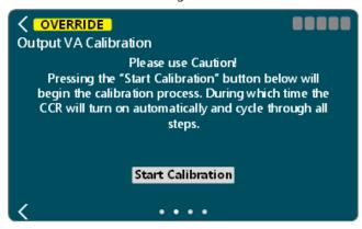
During calibration, the user will be given the ability to cancel the calibration operation, if necessary.
