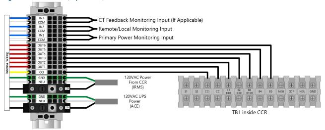
Figure 19: CSS wiring using IO Backplane
