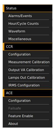
The menu will allow the user to navigate away from the main screen to various status and config screens. It is broken down into three sections "Status", "CCR", and "ACE". Under each section will be screens related to the section title.
