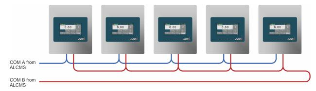
Using the recommended Belden 9842, the communication should be terminated using the example below.
