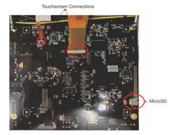
The MicroSD memory card, on the back side of the board, contains all the software for the ACE3. If an failed ACE3 unit is replaced, the MicroSD card can be removed from the failed ACE3 and placed in the new ACE3. See Figure 1.
