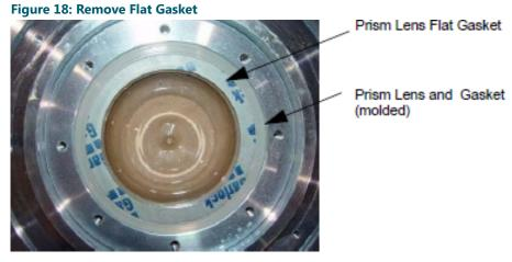
4. Turn the top cover over and push the prism lens and gasket out of the recessed pocket from the outside of the top cover.
