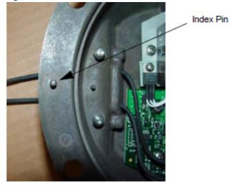
3. Gently put the inner cover over the top cover and align the index pin on the inner cover flange with the index pin hole in the flange of the top cover. Make sure that LED Power Cordset does not get damaged when the inner cover is installed on the top cover.
