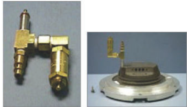
In-pavement Pressure Test Application
