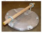
The lifting tool can be made from two  $1/2 \times 13$  eyebolts (1-inch ID) and a 1/2-inch diameter, 16-inch (406mm) long rod or pipe inserted through the eyebolts.
