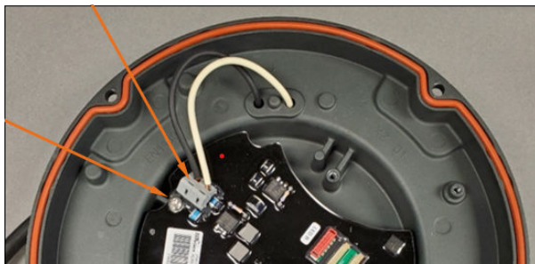
Figure 52: Locking secondary cables
