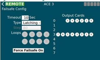
The button at the bottom can force failsafe on and off even if the ACE 3 is not in a failsafe situation.
