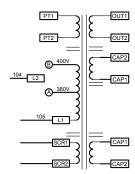
Figure 48: Internal Wiring Schematic (T4)
