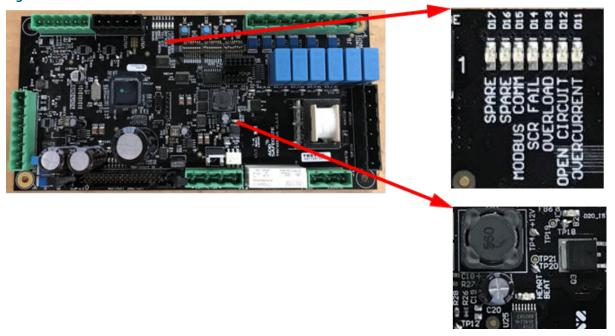
**Table 20: Diagnostic LEDs on the Control Board**
