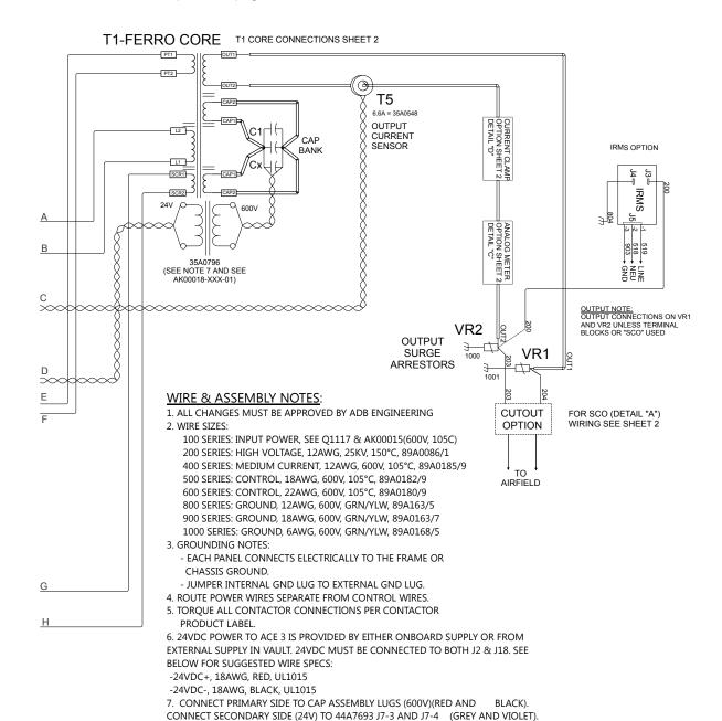
Figure 44: Internal Wiring Schematic (ACE3)
