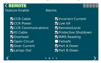
Disabling an alarm or warning prevents that alarm/warning from showing up on the alarm page and the corresponding event(s) will not be generated.
