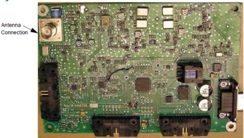
See Figure 3. The Control Board functions as the receiver, decoder, timer and central processor for the Radio Control Equipment.
