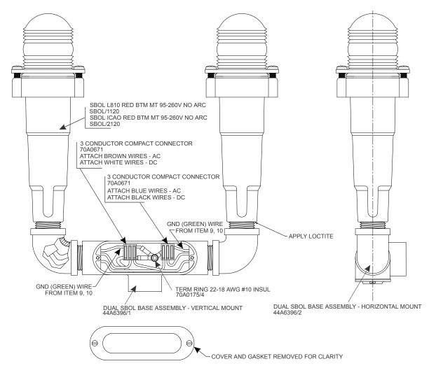
L-810(L) SBOL - Steady Burning LED Obstruction Light Parts
