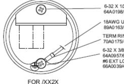
6-32 X 1/2 PAN HD PHIL 410 S.S. 64A0198/8/410 18AWG UL1015 16/30 GRN/Y 89A0163/7 TERM RING 22-18AWG #10 INSUL 70A0175/4 6-32 X 3/8 PAN HD PHIL 410 S.S. 64A0957/6/410 #6 EXT LOCK WASHER 66A0039/4
