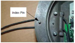
Figure 27: Index Pin of Inner Cover Flange
