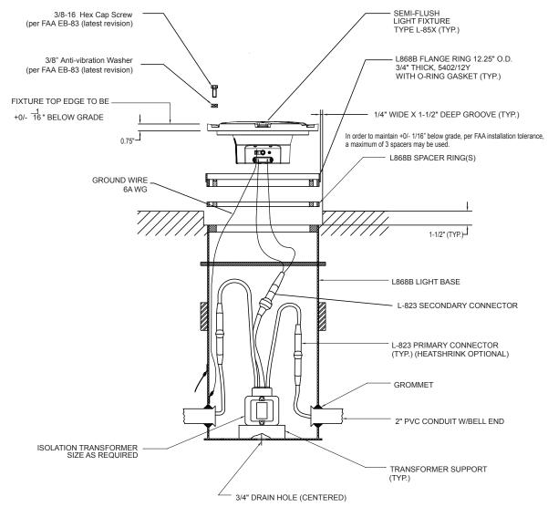
1. Torque according to: FAA EB-83 (latest revision).
