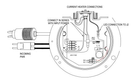
Figure 18: Wiring for 44A7281-1X
