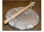
The lifting tool can be made from two 1/2 x 13 eyebolts (1-inch ID) and a 1/2-inch diameter, 16-inch (406mm) long rod or pipe inserted through the eyebolts.
