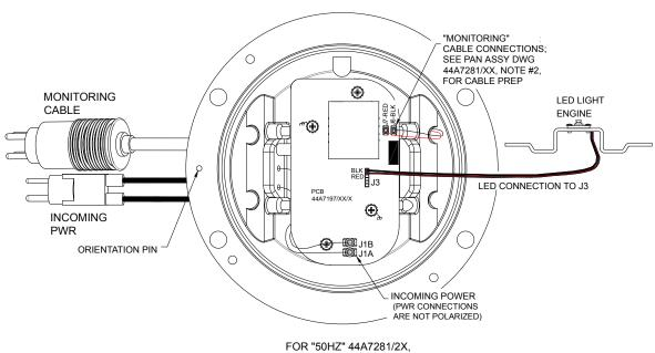
FOR "50HZ" 44A7281/2X, USE PCB 44A7197/50/X (NO SHUNT REQ'D)
